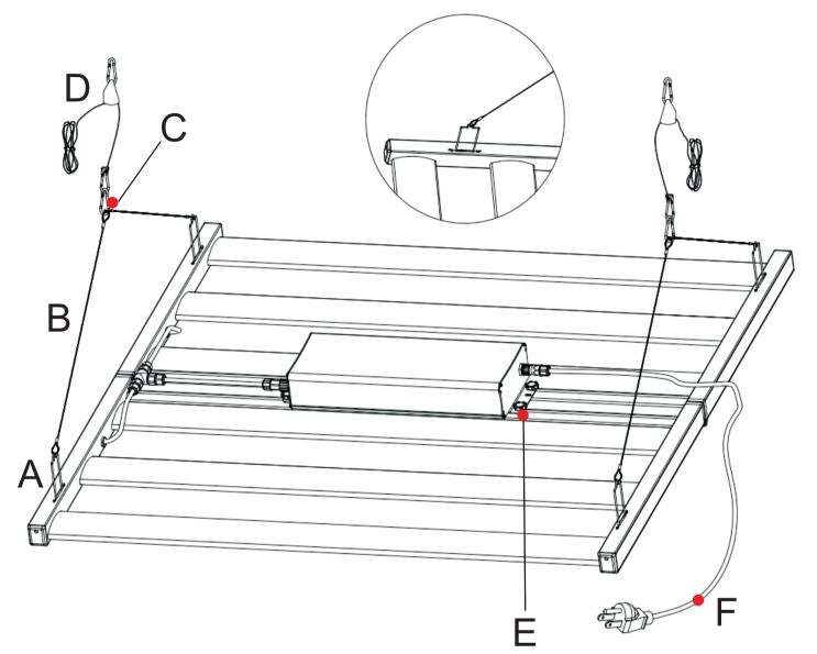
A: Mounting Clips (4 pcs) B: 21.26'' (54cm) Stainless Steel Ropes (4 pcs) C: Mounting Hooks (2 pcs) D: Adjustable Ratchet Hangers (2 pcs) E: Konb screws for Fixing LED Driver Box (4 pcs) F: AC Power Cord and Plug (1 pc)
