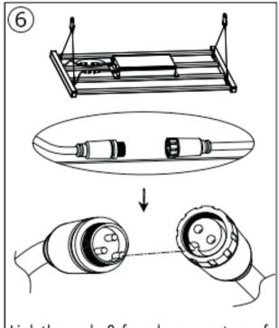
Link the male & female connectors of DC cables and twist them tightly.
